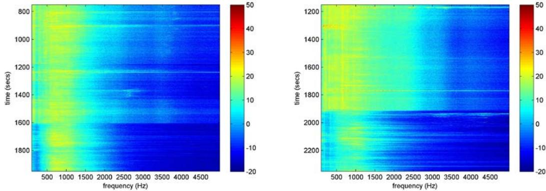
Figure 3: Frequency spectrum for T1 (left) and V27 (right). Turbines turned off at approx. 1600 respectively 1900 sec.
