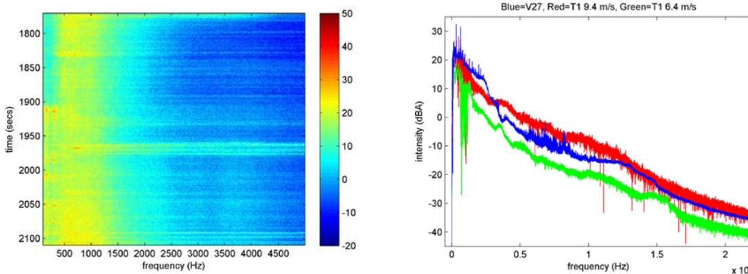
Figure 6: The frequency spectrum for the 9.4 m/s recording of the T1-turbine (turned on at approx. 1900 sec) and a comparison between the frequency distribution with background noise subtracted for the 6.4 m/s (green, lowest) and 9.4 m/s (red, highest for most frequencies) recordings for the T1-turbine as well as the V27 recording (blue, highest for low frequencies).
