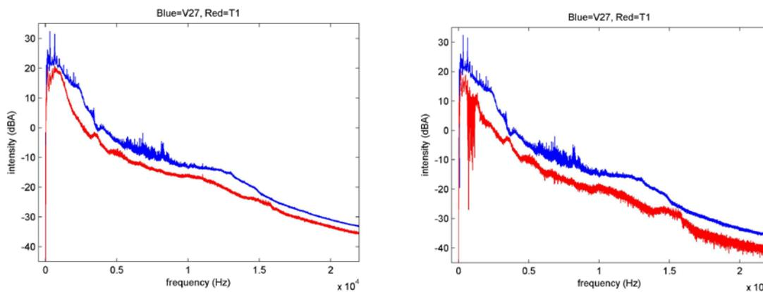
Figure 5: Comparison between T1 (red, lower) and V27 (blue, higher) regarding total noise (left) and turbine noise with background subtracted (right)
