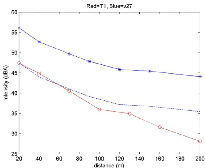
Figure 7: Noise propagation between T1 (red <sup>o</sup>) and V27 (blue \*) turbines. Dashed blue line is the blue line projected for comparison
